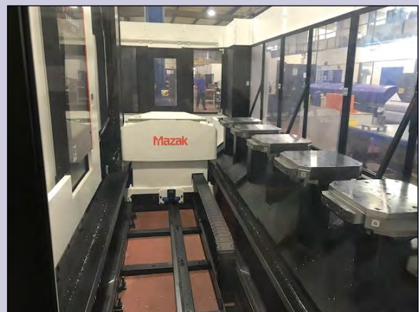
Yamazaki 5 Axis Machining Centre with Pallettech loading system
