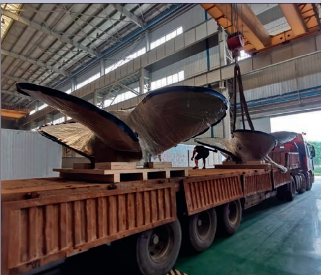
New Arctic Class 3 propellers for the Canadian Coast Guard
